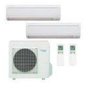
In a mini split system, the outdoor unit that is placed outside the house is connected to the indoor unit which is mounted inside your home by a set of piping and wiring systems that are usually passed through a small hole in the wall (usually just a 2 ½-inch hole or a 3-inch hole), linking both units as one single system. The pipes are usually the cooper
